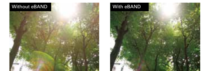
Tamron's eBAND coating effectively prevents mirror images that can occur in back lit photographs as a result of reflections on the lens surfaces inside the lens.
